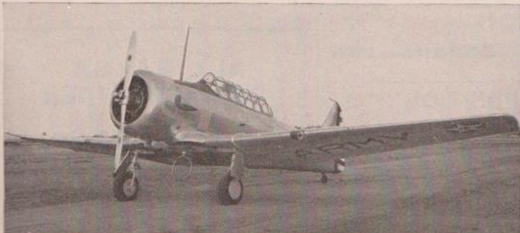
The North American AT-6 advanced trainer with retractable landing gear and radial engine. The crew is enclosed in this type
