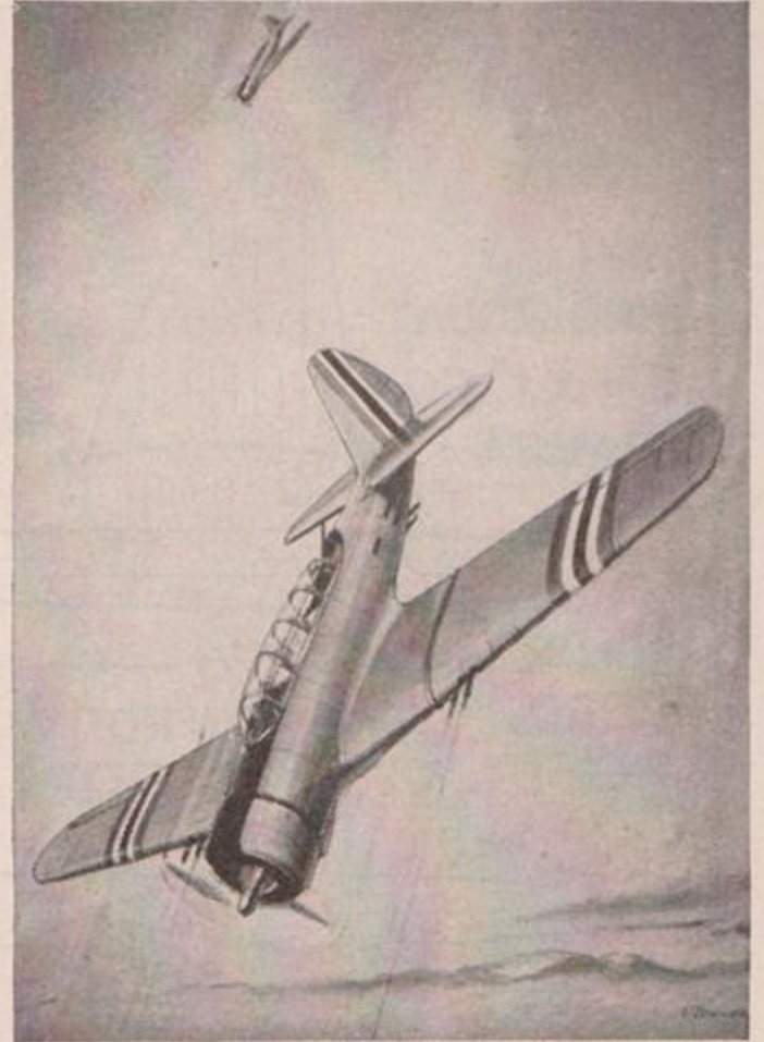
How the latest Northrop fighter N-3 will appear. It mounts five machine guns, one cannon and carries 2000 lbs. of bombs. Its high speed is 306 m.p.h.
