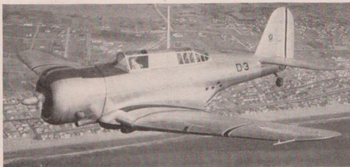
The 1200 hp. Douglas 8A-5 attack-bomber flying under Norwegian colors
